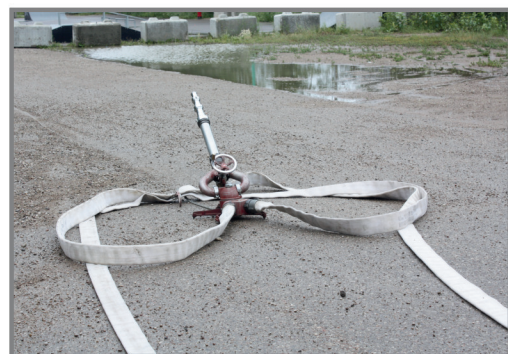
A portable monitor sits on the ground and can be moved where needed. It is safely secured, and hose lines are connected to supply water to monitor.
