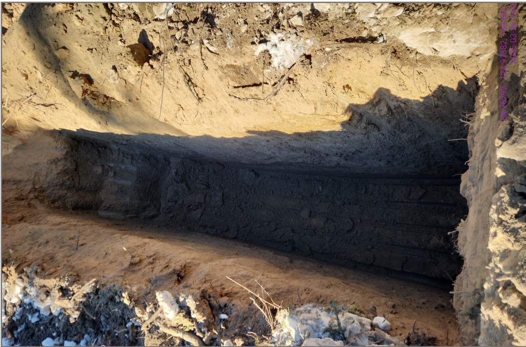
Photo 14: Borrow Source BS899, Testpit TP25-BS899-05 Fine-Grained Sand observed in Testpit TP25-BS899-05 (Photo Date: March 26, 2025)
