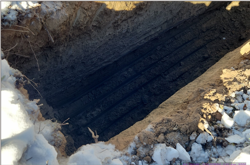
Photo 12: Borrow Source BS899, Testpit TP25-BS899-04 Fine-Grained Sand observed in Testpit TP25-BS899-04 (Photo Date: March 26, 2025)
