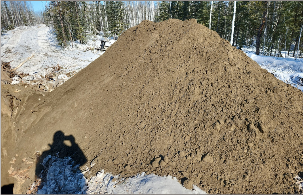
Photo 9: Borrow Source BS899, Testpit TP25-BS899-03 Fine-Grained Sand recovered from Testpit TP25-BS899-03 (Photo Date: March 26, 2025)
