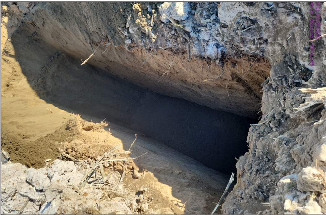
Photo 8: Borrow Source BS899, Testpit TP25-BS899-02 Fine-Grained Sand observed in Testpit TP25-BS899-02 (Photo Date: March 26, 2025)
