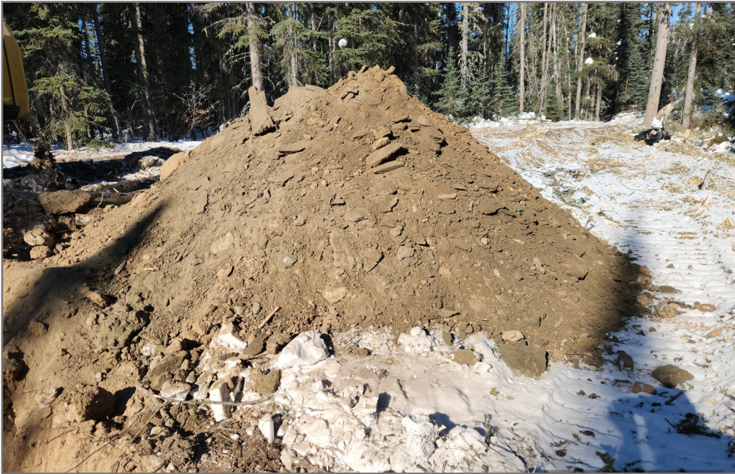
Photo 13: Borrow Source BS899, Testpit TP25-BS899-05 Fine-Grained Sand recovered from Testpit TP25-BS899-05 (Photo Date: March 26, 2025)
