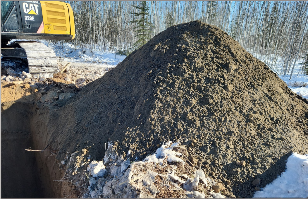
Photo 7: Borrow Source BS899, Testpit TP25-BS899-02 Fine-Grained Sand recovered from Testpit TP25-BS899-02 (Photo Date: March 26, 2025)
