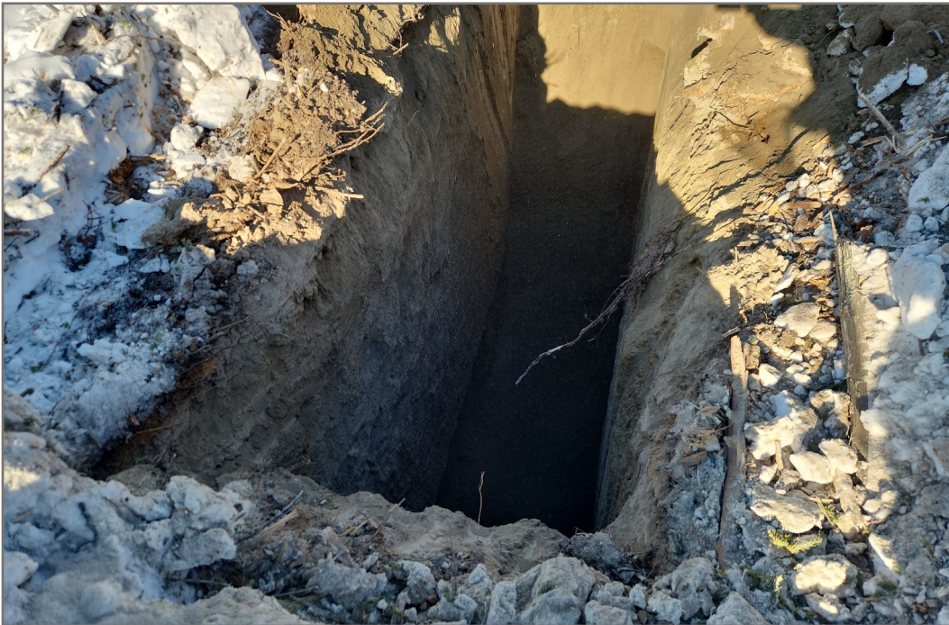
Photo 10: Borrow Source BS899, Testpit TP25-BS899-03 Fine-Grained Sand observed in Testpit TP25-BS899-03 (Photo Date: March 26, 2025)
