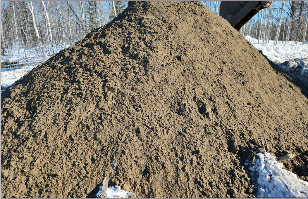
Photo 5: Borrow Source BS899, Testpit TP25-BS899-01 Fine-Grained Sand recovered from Testpit TP25-BS899-01 (Photo Date: March 26, 2025)
