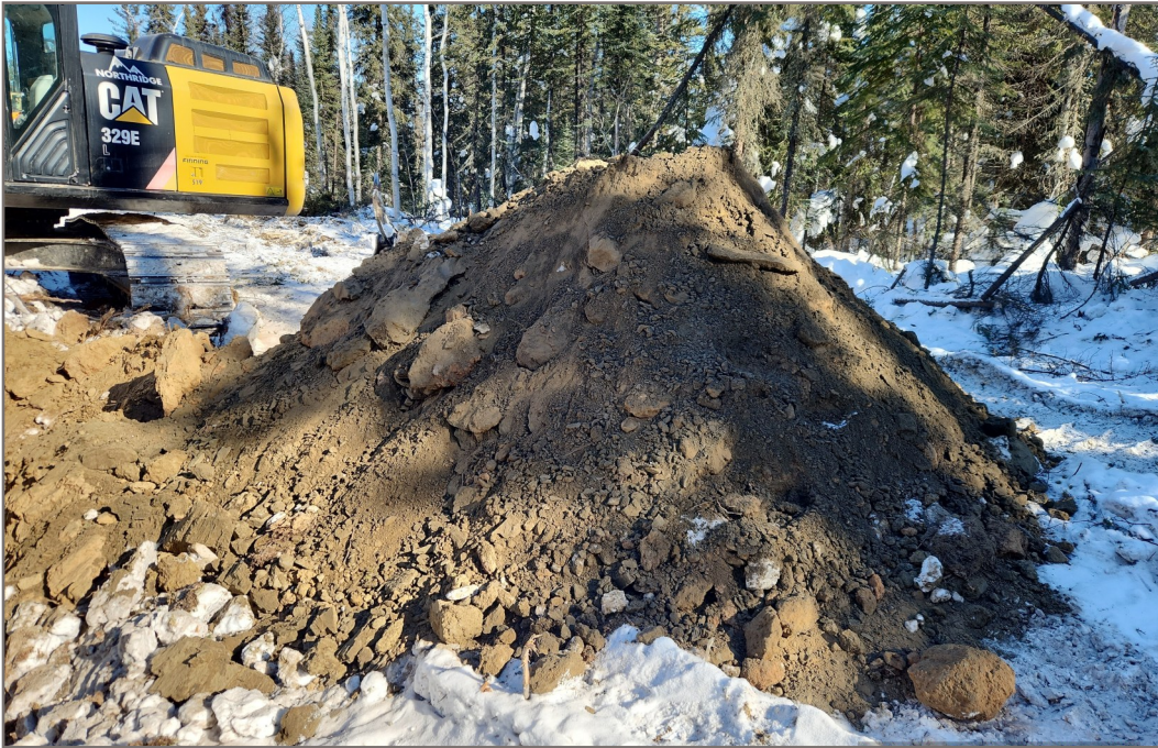
Photo 11: Borrow Source BS899, Testpit TP25-BS899-04 Fine-Grained Sand recovered from Testpit TP25-BS899-04 (Photo Date: March 26, 2025)
