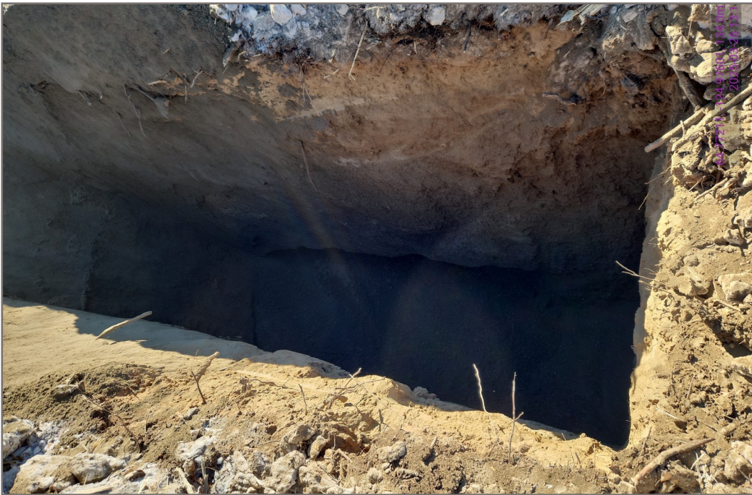
Photo 6: Borrow Source BS899, Testpit TP25-BS899-01 Fine-Grained Sand observed in Testpit TP25-BS899-01 (Photo Date: March 26, 2025)
